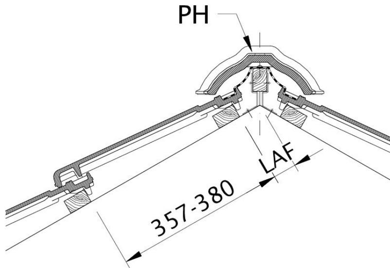
Drawing RATIO distance from batten to ridge intersection point, ridge batten spacing LAF
